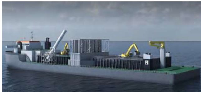
Figure 2 Placement of rock for pipe and cable crossings
