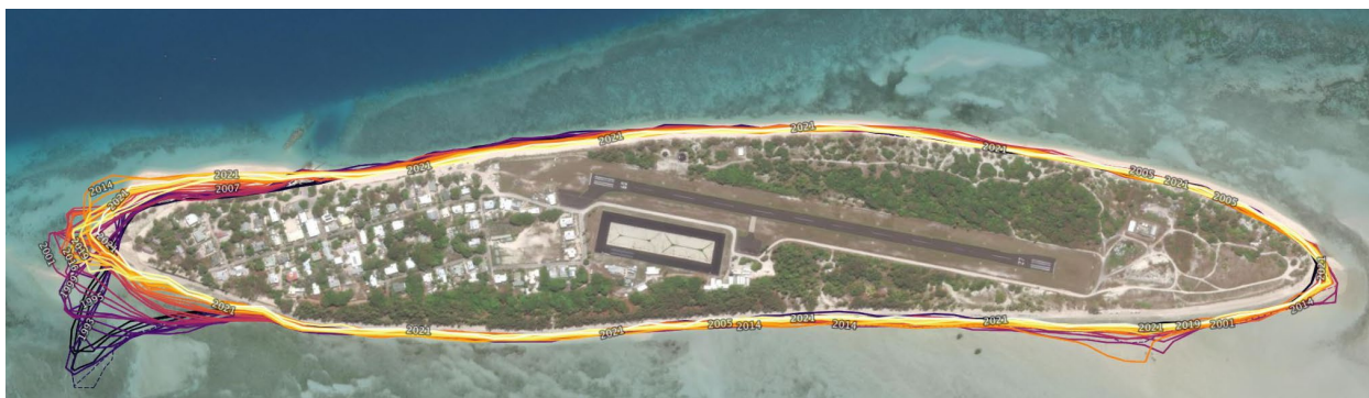
Figure 38 Foreshore locations captured over 30 years reveal significant changes in the foreshore location on Poruma's western end as a result of an imbalance in morphological processes. Note north and south coasts anchored by beach rock.
