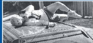
“This throw distance and angle is critical and together with the trajectory indicates the vehicle was travelling at speed prior to impact... The impact speed of the vehicle was... likely to be in the range of 40km/h to 50km/h.”
